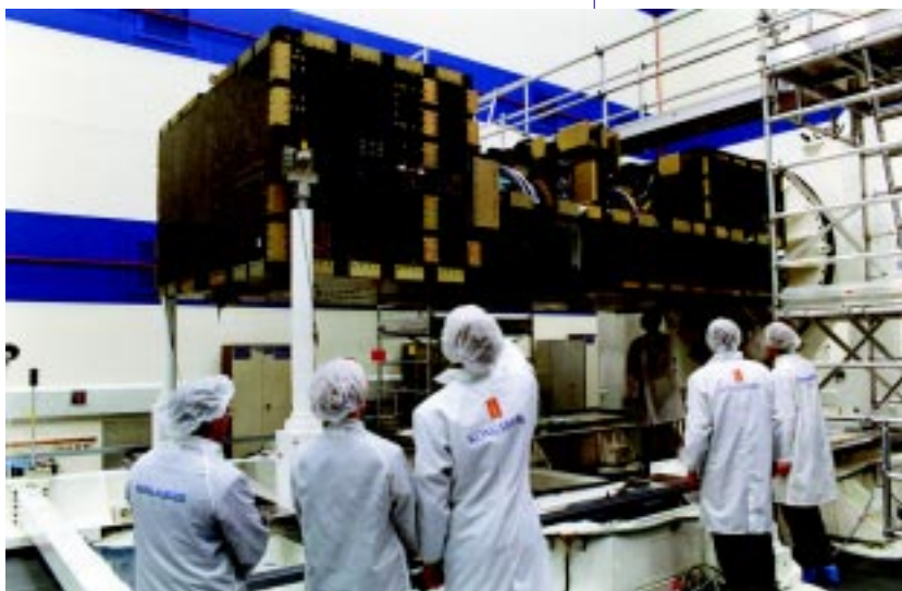
Structural Model of the ENVISAT Payload Carrier
