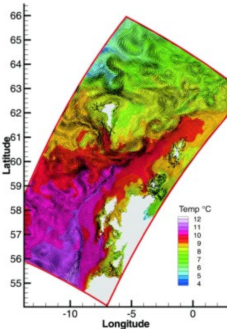
**Figure 2:** Model prediction of the ocean currents and sea surface temperature west of Scotland. Satellite based information on the sea surface temperature and ocean circulation fields are assimilated in to the ocean model, resolving the meso-scale ocean circulation structures.
