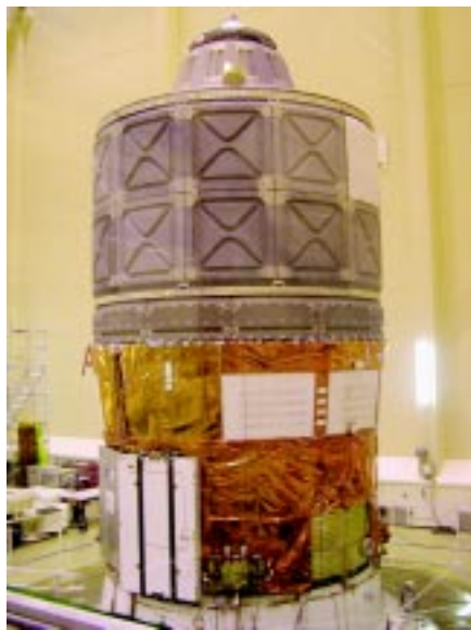
The ATV Structural Thermal Model (STM) is standing on the vibrator table.
