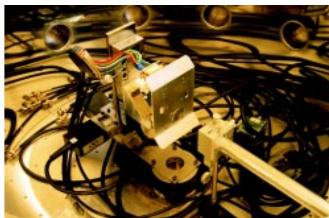
XSM flight model attached in a turnable arrangement inside a small vacuum chamber at the Department of Physical Sciences, University of Helsinki. This is the facility specially built for XSM ground calibrations. With accurate adjustment of position and attitude of the detector with respect to the incoming X-ray beam, the arrangement enables measurements of the detector response and effectivity over the full field-of-view of XSM.
