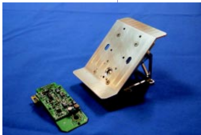
XSM flight model with the final design, and the front end electronics board separated. The enlarged front plate of the sensor box was designed for additional passive cooling of the system due to the very demanding thermal requirements of SMART-1 mission.
