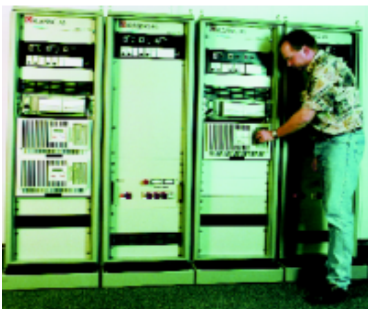
Technicians work with the Electronic Ground Support System, a test system for satellites.
