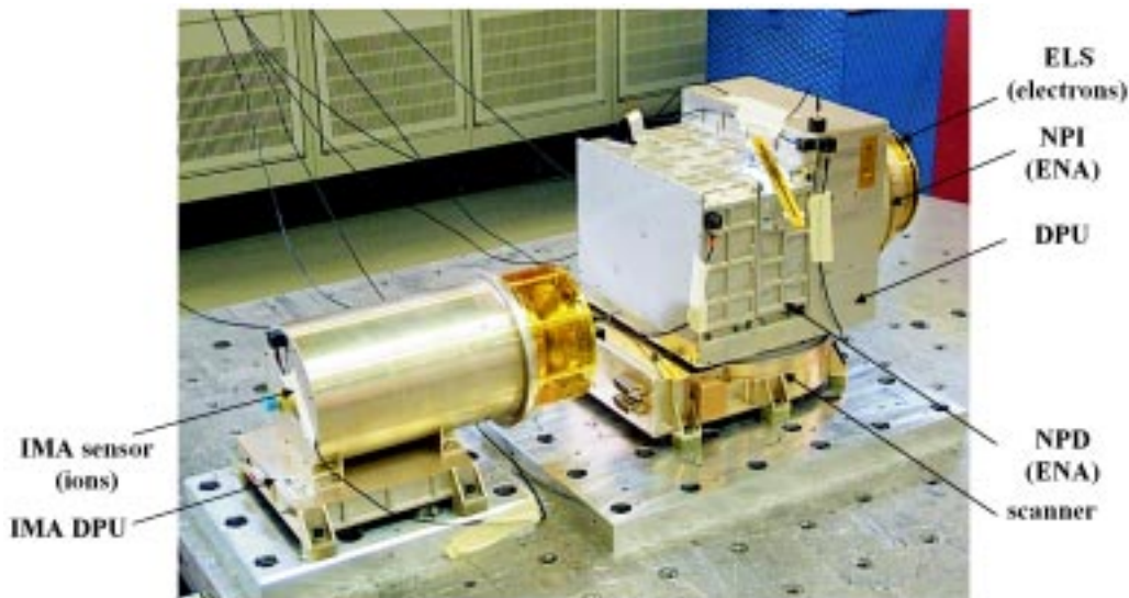
Figure 2. The main unit (to the right) and IMA with all four sensors, and digital processing units (DPUs) marked.
