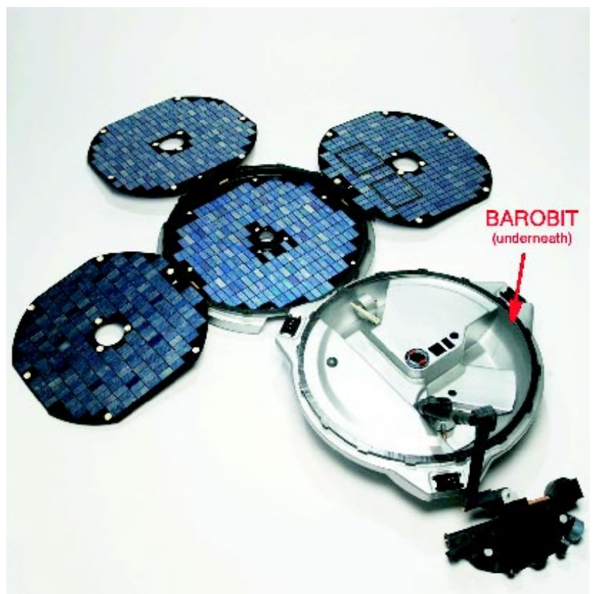
Barobit pressure device mounted onboard the Beagle 2 landing vehicle ( http://netlander.fmi.fi/BAROBIT/ )
