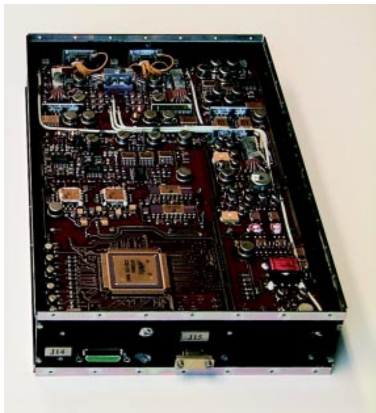
Figure 3. The LAP electronics boards mounted in their frame, ready for intergration with the RPC main unit. The frames from four RPC instruments together form the main RPC electronics box. The board seen contains the analog electronics, with the digital board invisible beneath.
