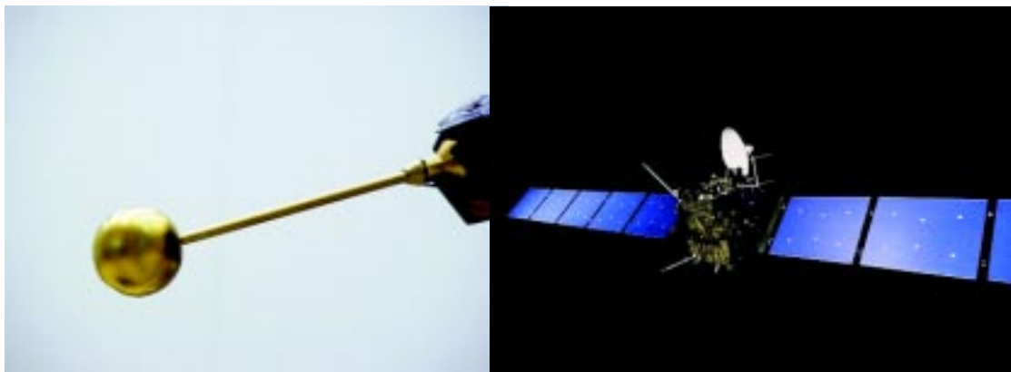
Figure 2. Rosetta in space (at right), with solar panels and booms deployed. The two booms, extending to the upper and lower left from the spacecraft, hosts some of the sensors of the RPC, a package of plasma instruments. At the boom tips, the Langmuir probes of the LAP instrument, one of which is shown in detail in the left panel, will provide the density, temperature and flow speed of the plasma environment. Unlike most instruments onboard, the RPC can gather useful science data immediately soon after launch, by measuring the properties of the solar wind and the environments of Earth and Mars when Rosetta passes these planets.
