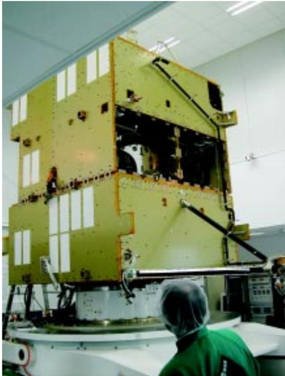
The Finnish company, Patria Finavitec Oy, supplies the main structure of the satellite. The company is responsible for the structural design, manufacture, assembly, integration and static testing. The order was an important milestone for the Finnish company, as it was the first time the company was responsible for the design and manufacture of the whole structure of a spacecraft.
