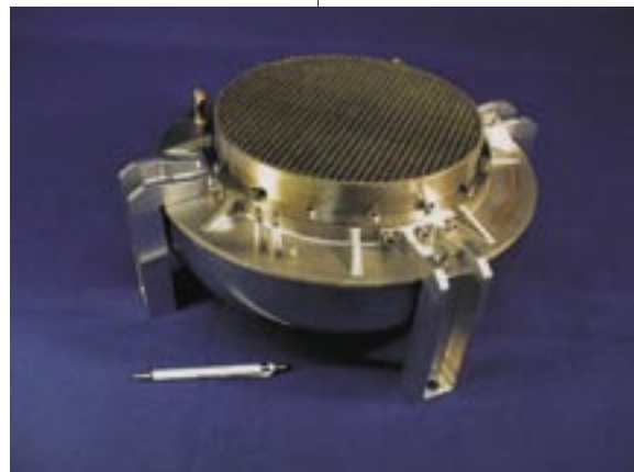
The JEM-X microstrip detector package, designed and fabricated of Metorex International Oy.
