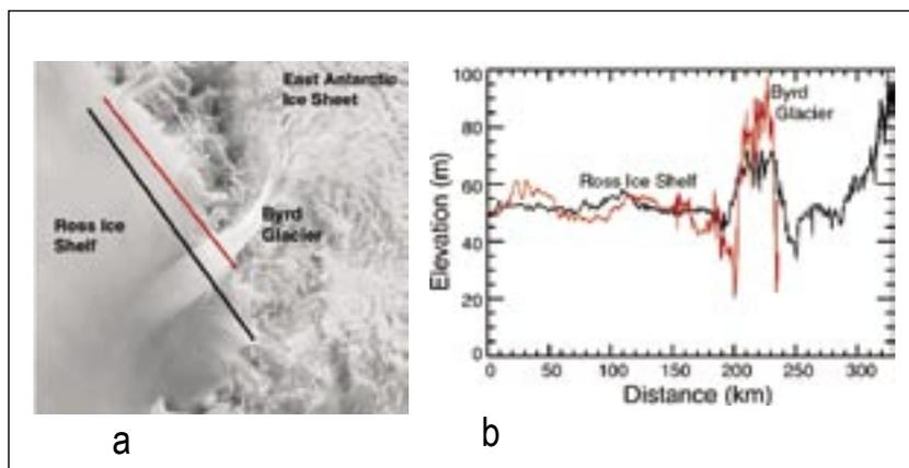
Figure 4. a) RADARSAT image of the Byrd Glacier in Eastern Antarctica with two IceSat profiles superimposed; b) IceSat elevation measurements across the Byrd Glacier (Courtesy: NASA).
