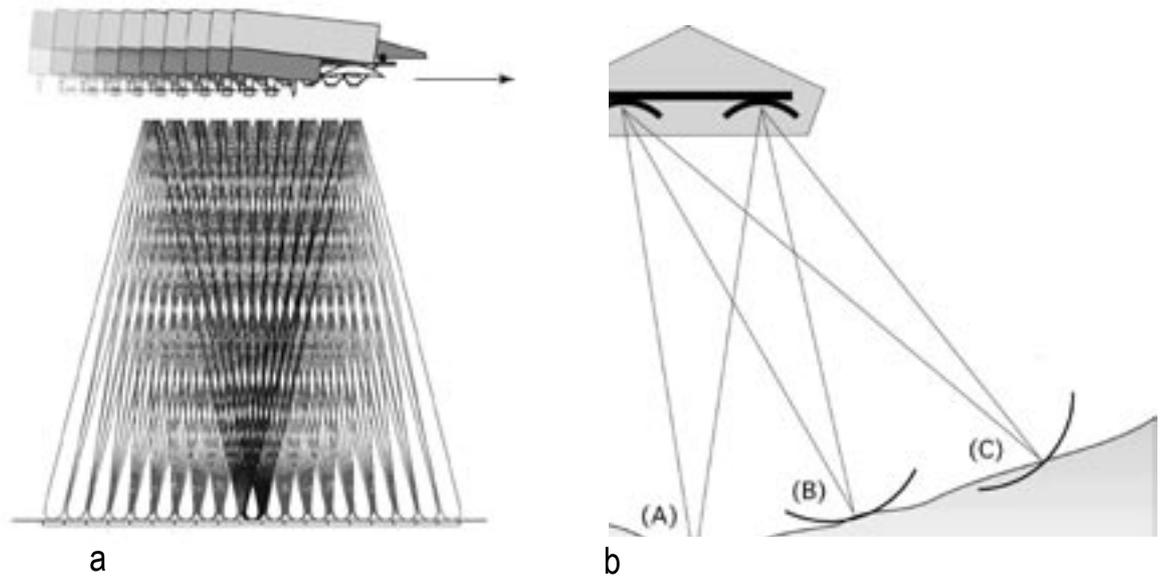
Fig. 3. Principle Operation Modes of the SIRAL altimeter. a): SAR-Mode over sea ice, where the arrow shows the flight direction. b): SARIn-Mode over steep ice sheet terrain, showing the capability to measure across track slope of the terrain.
