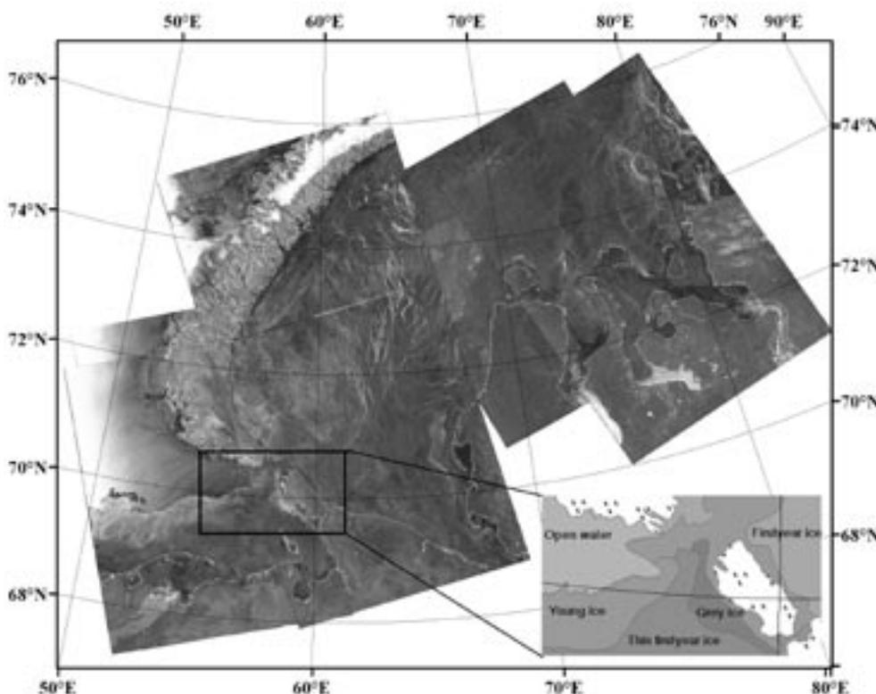
*Figure 1. Mosaic of ENVISAT ASAR Wideswath images obtained on 27 – 28 February 2005, showing the ice extent, ice types, leads and polynyas which are important for ice navigation. The inserted ice chart is based on analysis of a part of the mosaic covering the Kara Gate area.*
