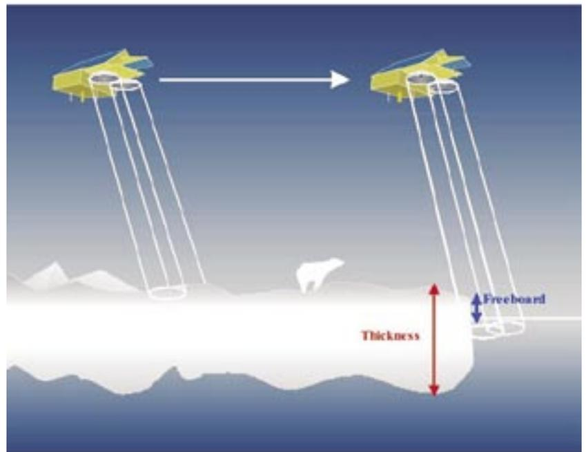
Figure 2. Illustration of CryoSat measurements over sea ice. The freeboard height will be retrieved by estimating the height difference between ice floes and open water.
