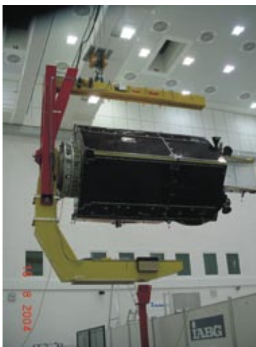
Figure 5. CryoSat during mass properties testing at IABG in Munich (courtesy Thomas Usbeck, EADS Astrium GmbH). The three Terma Star Trackers are mounted on the SIRAL bench shown to the right. Using three Star Trackers guarantees not only redundancy, but also the possibility of having multiple camera's tracking simultaneously independently of potential sun and/or moon blinding.
