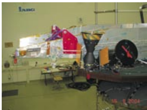
Figure 3. Two of the three Terma Star Trackers mounted on the CryoSat SIRAL bench (courtesy Thomas Usbeck, EADS Astrium GmbH). Low operational camera CCD temperature obtained by the use of forward looking radiators ensures not only high accuracy due to lower image noise but also longer operational lifetime. The primary Star Tracker degradation factor in-flight is the proton bombardment in-orbit. For CryoSat this mainly happens during passages through the South Atlantic Anomaly and the poles especially during solar eruptions. The proton degradation will be mitigated by the low operational CCD temperature and the use of robust software algorithms.
