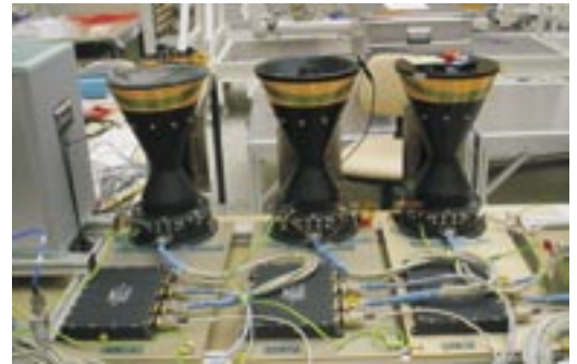
Figure 1. The CryoSat Terma Star Trackers during integration testing at EADS Astrium GmbH (courtesy Thomas Usbeck, EADS Astrium GmbH). The three camera heads in the background are mounted onto their thermo-mechanical stable brackets. Straylight rejection baffles are mounted on top of the brackets. The Star Tracker data processing units visible in the foreground are mounted in satellite body. Note that a star field simulator is mounted inside the middle baffle. This simulator offers a very accurate optical stimulus for the Star Tracker in test enabling complete test of all software modes such as initial acquisition (lost-in-space) and tracking. Testing with the star field simulator requires no special test mode being implemented in the Star Tracker software and can thus also be used during last minutes testing prior to launch.
