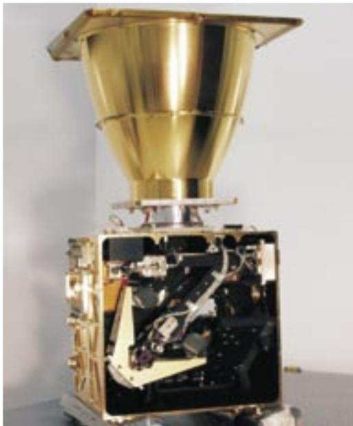
*The Fourier Transform Spectrometer is the primary instrument selected for the ACE mission onboard the SCISAT satellite. This picture shows the input optics side of the instrument. The ACE-FTS was built by ABB Bomem, located in Quebec City. (Photo: Canadian Space Agency, ABB Bomem)*
