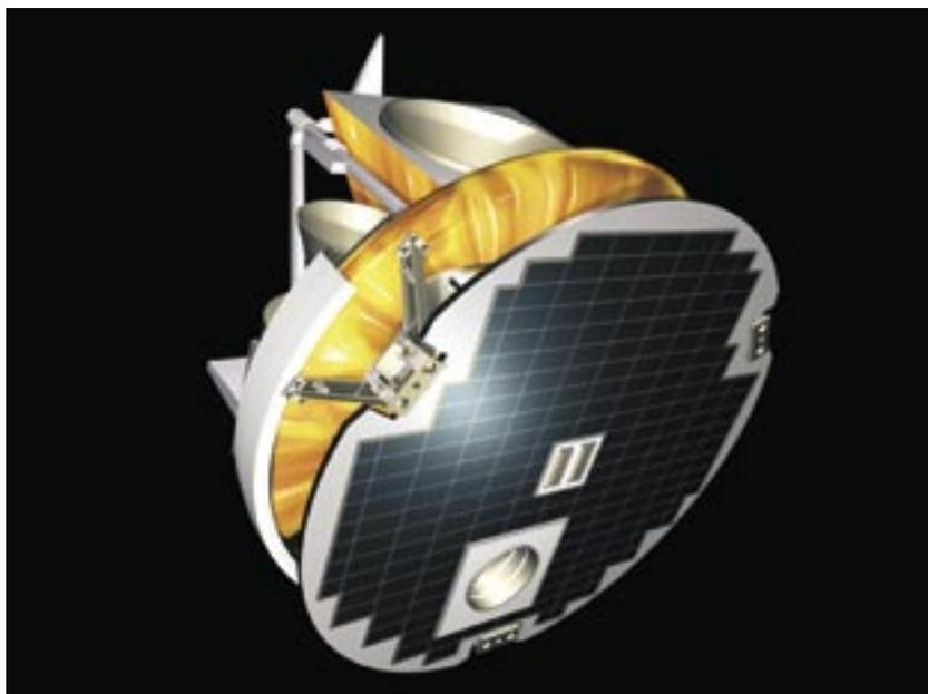
SCISAT is tiny compared to giant satellites such as RADARSAT-1: it is 112 cm in diameter, 104 cm high, and weighs only 150 kg. Though small, this satellite is very powerful. Its size contributes to the cost-efficiency of the mission and, as such, is a model for future small satellite missions.
