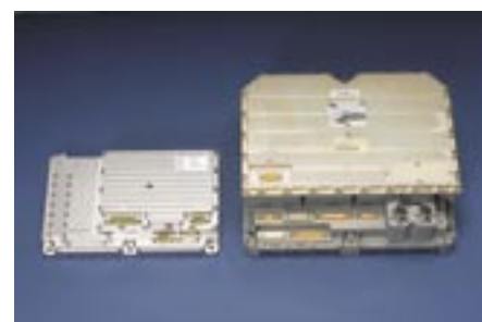
Guidance & Control Computers for Vega and Ariane 5. Higher performance with lesser weight for the new version.
