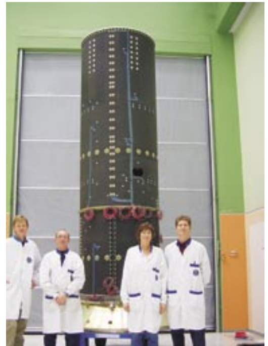
The central cylinder for Spacebus 3000 ready for qualification test at the Linköping plant. Photo: Saab Ericsson Space
