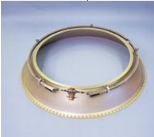
Adapter and separation system for satellites. Photo: Saab Ericsson Space
