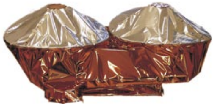
The Siral Antenna assembly is dressed for launch. The MLI (golden) and the sunshield (grey) have been fitted and manufactured by Austrian Aerospace in Vienna.
