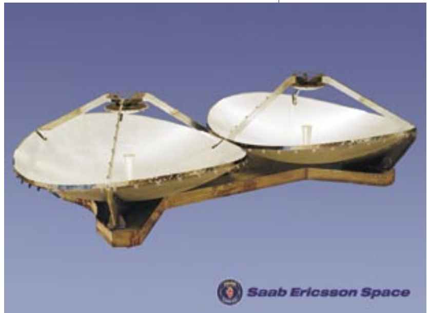
The overall size of the Siral antenna assembly is 2.3 x 1.7 x 0.7 m and the total mass without thermal blankets is 31kg. Three star-trackers will be mounted on the other side of the base-plate facing space.
