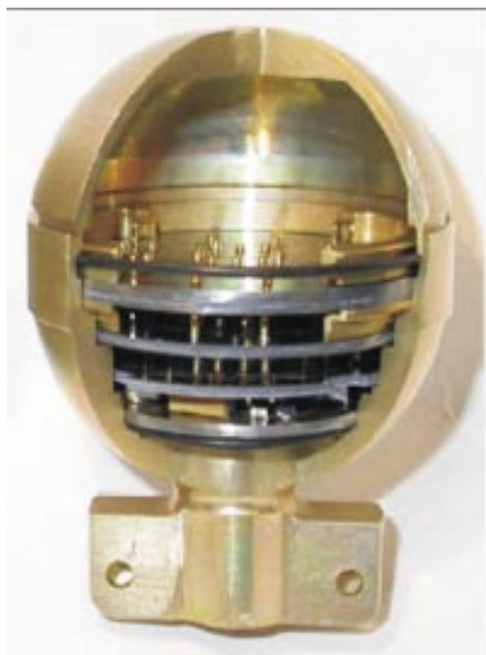
Microthruster pod with 4 thrusters along the "equator". Photo: SSC
