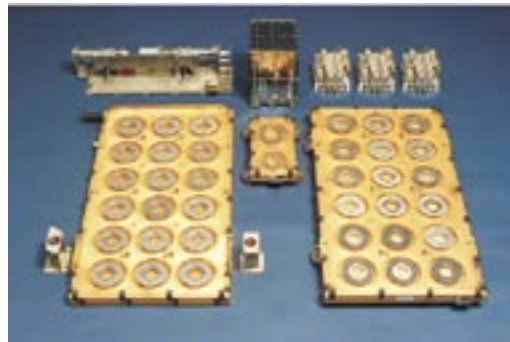
Antenna for the GRAS Radio occultation instrument, developed and built by Saab Ericsson Space. Photo: Saab Ericsson Space
