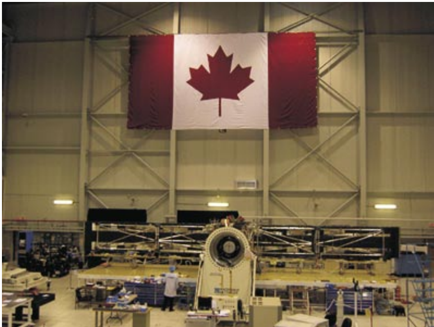
The backside of the SAR antenna in the integration hall. Photo: Canadian Space Agency.
