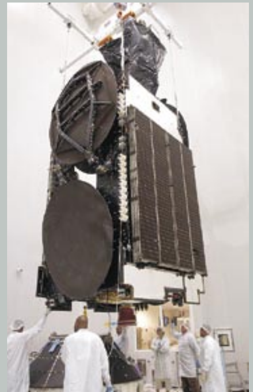
A large communication satellite ready for launch. One can see the apogee engine nozzle at the bottom. Photo: ESA/CNES/ARIANESPACE
