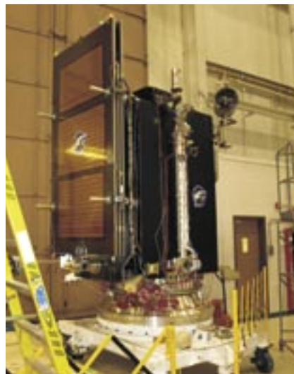
An engineering model of LRO outside the clean room. The folded solar arrays are visible on the left side of the satellite.
