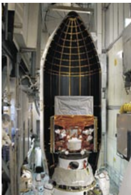
The last preparations before launch of GLAST. The picture is taken at the launch pad, and the first half of the fairing is already at the right place. Photo: NASA/ Goddard.
