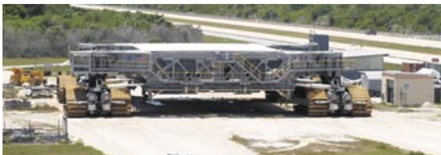
The Crawler. A very especial vehicle, designed for transport of Saturn 5, used for the Space Shuttle and from 2015 possibly used for the new generation of American moon launchers.
